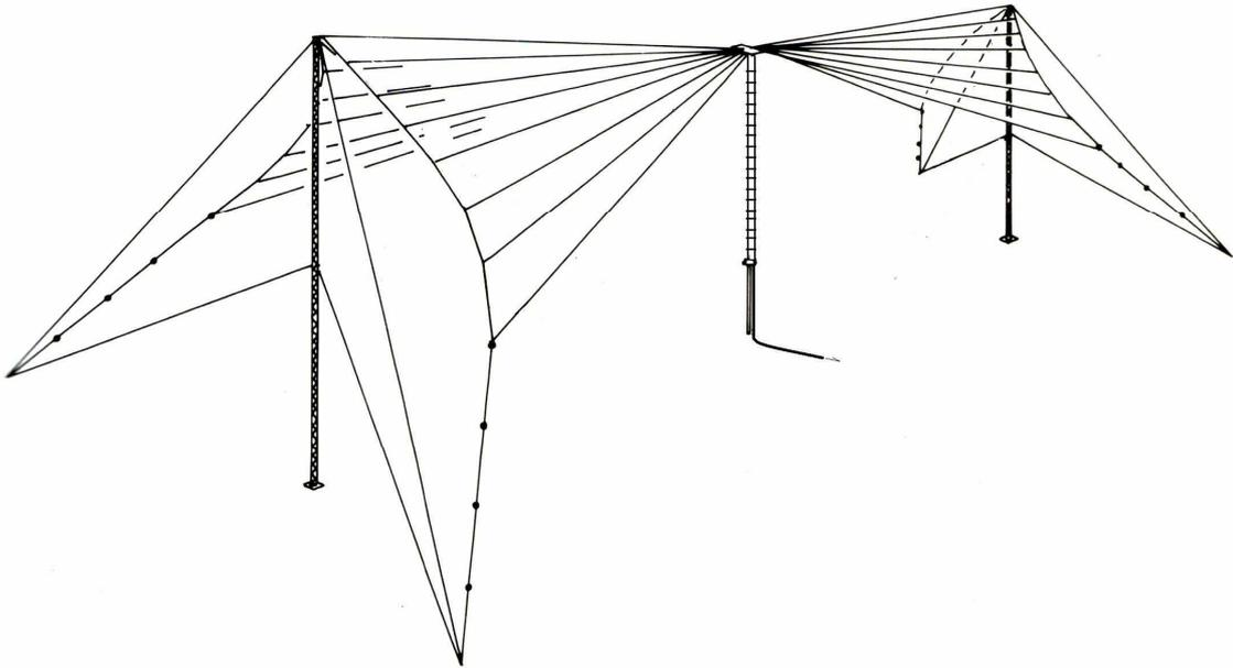
Our HF broadband Biconical Dipoles are highly efficient, horizontally polarised antennas that at lower frequencies are suitable for short to medium range communication and at the higher frequencies have the strongest signals at lower angles for long range propagation.
